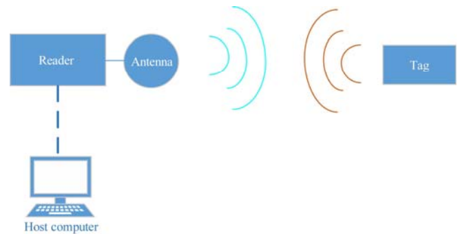
Figure 1 Architecture of a RFID system
